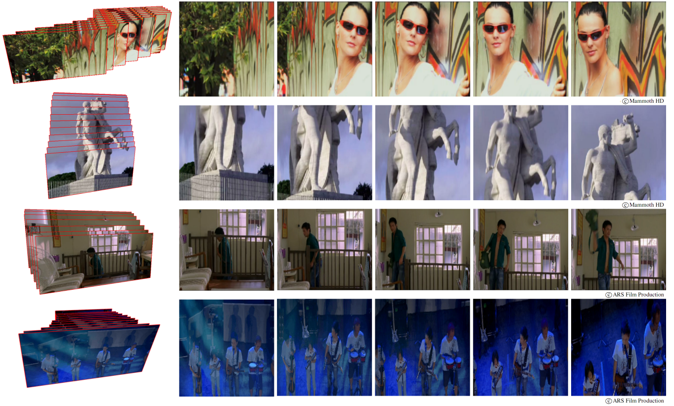
Figure 8: Left: frame alignment examples under different types of camera motions, consisting of sliding, yaw, pitch, and zoom motions. Right: the resized key frames. Note that the visually prominent features (e.g., human shapes and window shapes) are well preserved both spatially and temporally.
