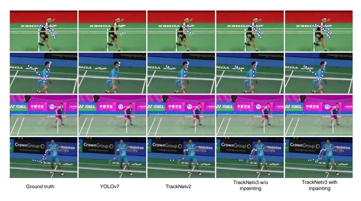
Figure 4: We conducted a comparative analysis of tracking results achieved using YOLOv7, TrackNetV2, and TrackNetV3, both with and without rectification modules. Each example portrays a video frame with previously tracked shuttlecock positions, which are represented by white dots surrounded by blue boundaries. As observed, YOLOv7 overlooked numerous shuttlecocks. Although TrackNetV2 demonstrated superior detection efficacy, it underperformed TrackNetV3.
