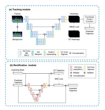
Figure 3: The network architecture of TrackNetV3. (a) The tracking module processes a sequence of video frames to produce respective heat maps, identifying the shuttlecock locations. (b) The rectification module refines shuttlecock trajectories by filling in erroneously detected shuttlecock positions.
