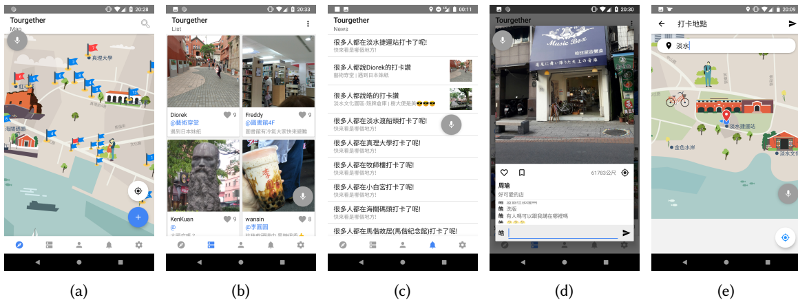
Fig. 3. System design of Tourgether, including (a) its GPS-enabled Tourist Map displaying graphics of important POIs and displaying check-ins with flag icons; (b) its News Feed page presenting all user check-ins; (c) all received notifications, divided into three categories, i.e., the most-liked current check-ins, the most checked-in areas, and newly checked-in POIs that the user has never visited; (d) its check-in post interface, with like, save and locate buttons below the image; and (e) its page for choosing a location when posting a check-in.
