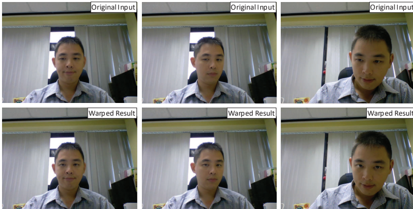
Fig. 10. Our system can dynamically estimate eyeball rotation angles to correct eye gaze. The participant is allowed to move his body and head poses during video conferencing.
