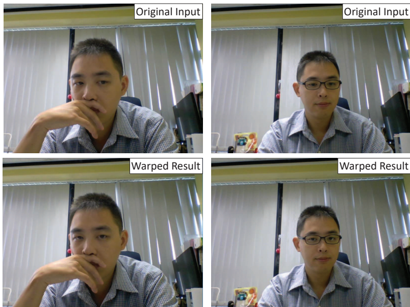
Fig. 11. Our system can correct eye gaze even when a participant's head is partially occluded by his or her hand or accessories such as eyeglasses.
