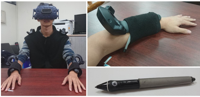
Figure 3: (Left) Participants equipped with HTC Vive controllers and trackers. (Top right) Controller strapped to arm and used in conjunction with inverse kinematics model to determine elbow joint position. (Bottom right) Plastic finger cushion on stylus for resting thumb.
