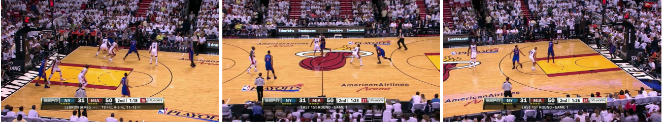
Fig. 5. Left to right: video frames captured in the left, middle, and right viewpoints. The slope of the top court boundary changes when the camera pans. We apply this characteristic to determine the viewpoint similarity between two video frames before tracking KLT features and computing the homography transformation.
