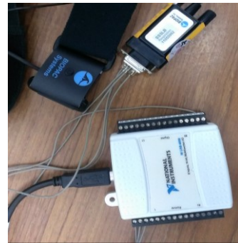
Fig. 2. Connection between SS5LB and NI USB-6009.
