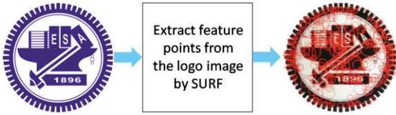
Fig. 7. An example of feature point detection using the SURF algorithm.
