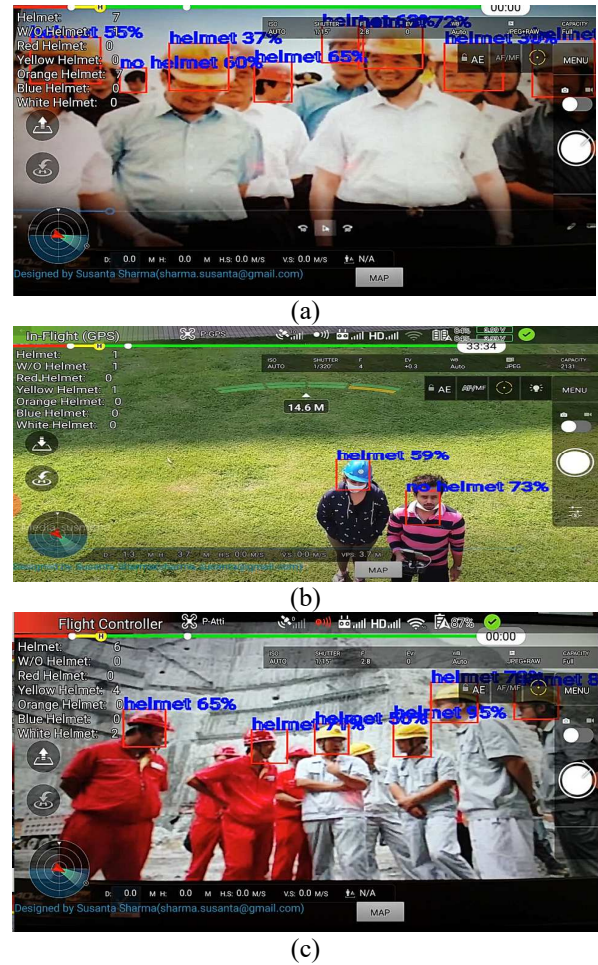
Fig 6. Three case scenarios for safety-helmet observation (a) Case 2, (b) Case 9, and (c) Case 10.
