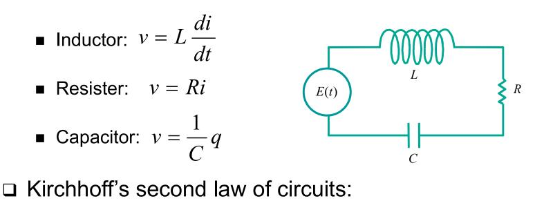
Voltage drop = Impressed Voltage, that is:
