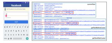
Fig. 12. Demonstration of the alternative deployment that runs the encryption service in an isolated process: the hijacked channel can only receive encrypted input texts.
