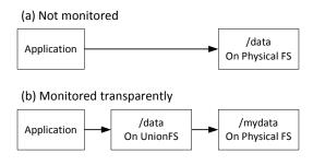
Figure 3 Access a real file system via a transparent intermediate layer.
