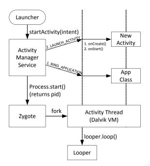
Figure 4 Android's application launch process.
