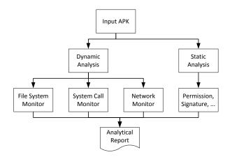
Figure 2 The components of an inspection instance.
