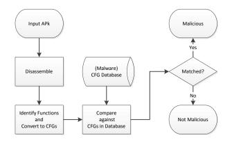
Figure 8 The malicious application detection flow of androguard.
