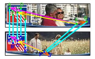
Fig. 4. Removing incorrectly matched key points from the images.
