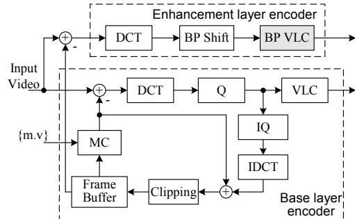
Fig. 1. The block diagram of MPEG-4 FGS encoder.
