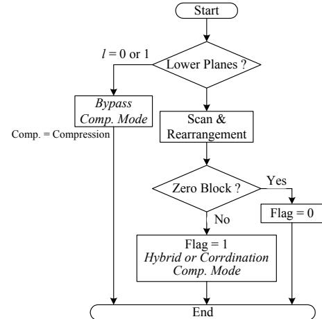
Fig. 3. Flow diagram of *adaptive bit-plane coding* scheme.
