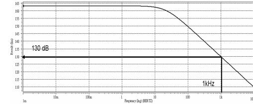
Figure 8. CMRR performance of the current-balancing IA.
